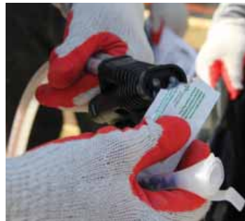
Application of petroleum jelly to spray gun
